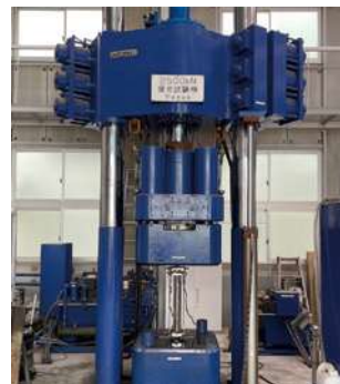
Elastic/plastic reversed cyclic test (SD490 D41)
